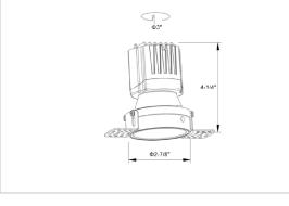
CRI >90 Beam Angle 15° Light Distribution Spot COB LED Type LED Light Source Osram SOLERIQ S 19 Start Time Instant Driver Stand Alone (included) **Operating Position** Non - Swiveling Type On-Off / Triac / 0-10 V Dimming Construction Round Mounting Type Recessed Single Head Heads **Body Material** Aluminium Die cast Finish White 4" Height 6-1/2" Diameter Cut Out 3" Darklight Technology Black, Silver Optics Application Area Guest Room, Corridor, Restaurant, Meeting Room Club, Hall, Hotel Entrance
